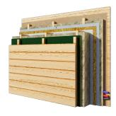
Section of the external walls with an internal drywall finish. Class A / A+:
